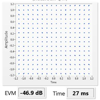
Figure 2. Typical Constellation Graph, EVM Measurement, and Measurement Time of an 802.11ac MCS9 Signal at 5.8 GHz.
